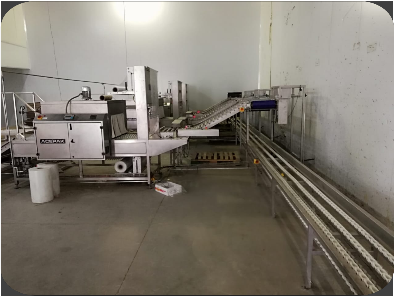
A conveyor that conveys Woven Poly bags from the Production to the Dispatching Areas
